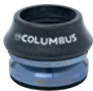
COMPASS CARBON CERAMIC ZV7STEERKITI 1-1/8" UPPER AND LOWER 45° CERAMIC ACB - CARBON TOP CAP STACK HEIGHT 16+0.7=16.7mm HEADTUBE O.D. Ø 46mm - HEADTUBE I.D. Ø 41.2mm
