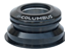
COMPASS 1.5" MTB 733SSSIX 1-1/8" UPPER, 1.5" LOWER 45° STAINLESS STEEL ACB - ALLOY TOP CAP STACK HEIGHT 10.1+2.8=12.9mm HEADTUBE O.D. Ø 50mm/61mm HEADTUBE I.D. Ø 44mm/54.9mm
