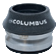
COMPASS CARBON ZV7STEERKITH 1-1/8" UPPER AND LOWER 45° STAINLESS STEEL ACB - CARBON TOP CAP STACK HEIGHT 16+0.7=16.7mm HEADTUBE O.D. Ø 46mm - HEADTUBE I.D. Ø 41.2mm
