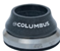
COMPASS 1.5" CARBON ZV7STEERKITF 1-1/8" UPPER, 1.5" LOWER 45° STAINLESS STEEL ACB - CARBON TOP CAP STACK HEIGHT 16+0.8=16.8mm HEADTUBE O.D. Ø 46mm/56mm HEADTUBE I.D. Ø 41.8mm/52mm
