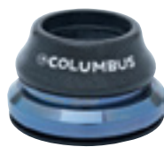
COMPASS 1.5" CARBON CERAMIC ZV7STEERKITG 1-1/8" UPPER, 1.5" LOWER 45° CERAMIC ACB - CARBON TOP CAP STACK HEIGHT 16+0.8=16.8mm HEADTUBE O.D. Ø 46mm/56mm HEADTUBE I.D. Ø 41.8mm/52mm
